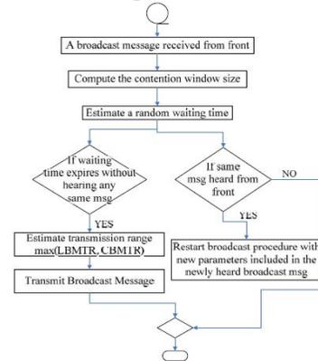
Fig. 4: Broadcast message forwarding procedure
