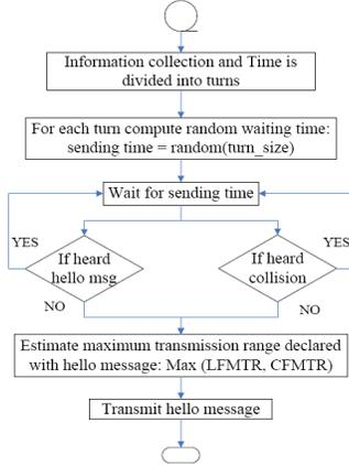
Fig. 2: Hello message sending procedure
