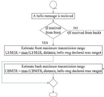
Fig. 3: Hello message receiving procedure
