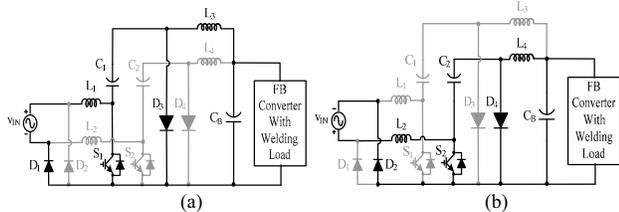
Fig.2. Operating circuits of the proposed BL Cuk converter based AWPS during positive and negative half-cycles of the supply voltage.
