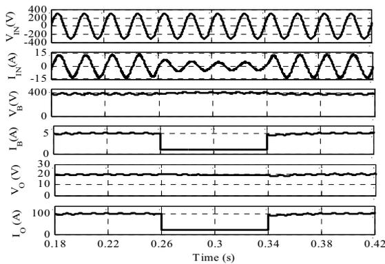
Fig.5. Dynamic performance of the proposed AWPS at 20% load.
