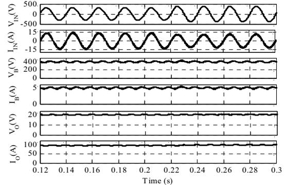
Fig.7. Dynamic performance of the proposed AWPS at  $V_{IN}$  of 170 V and full load condition.
