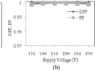
Fig.12. PQ indices of proposed AWPS under various supply voltage conditions. (a) Source current,  $I_{in}$  and its THD at different supply voltage conditions; (b) DPF and PF at different supply voltage conditions
