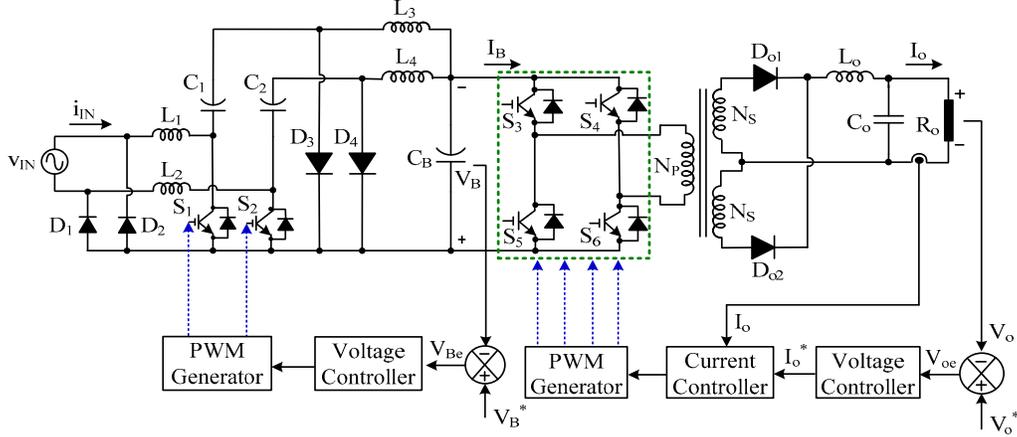
Fig.1. Schematic of BL Cuk converter and isolated FB converter based AWPS.
