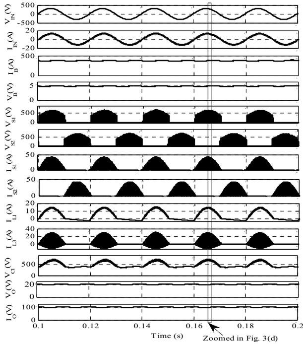
Fig.4. Steady state behavior of proposed AWPS at 220 V AC mains and 100% load.
