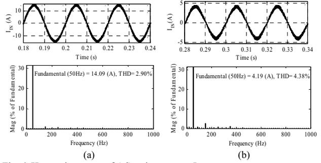
Fig. 6. Harmonic spectra of AC mains current,  $I_{IN}$  (a) at 220 V AC mains and 100% load; (b) at light load conditions
