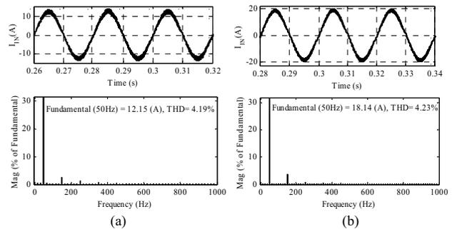
Fig.9. Harmonic spectra of AC mains current,  $I_{IN}$  (a) at 270 V AC mains and full load; (b) at 170 V AC mains and full load.
