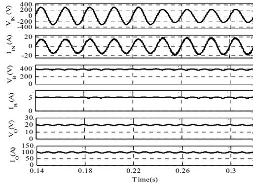
Fig.8. Dynamic performance of the proposed AWPS at  $V_{IN}$  of 270 V and full load condition.
