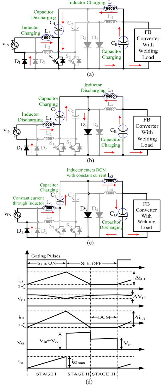
Fig.3. Operating stages of BL Cuk converter during steady state. (a) Stage I; (b) Stage II; (c) Stage III; (d) Waveforms during one switching period.
