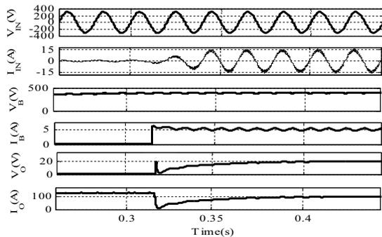
Fig.10. Dynamic performance of the proposed AWPS during over-current condition (i.e. transition from short-circuit to full load).
