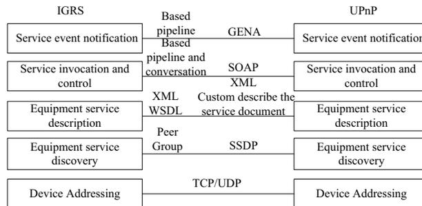
Figure1. Equipment interaction diagrams of IGRS and UPnP
