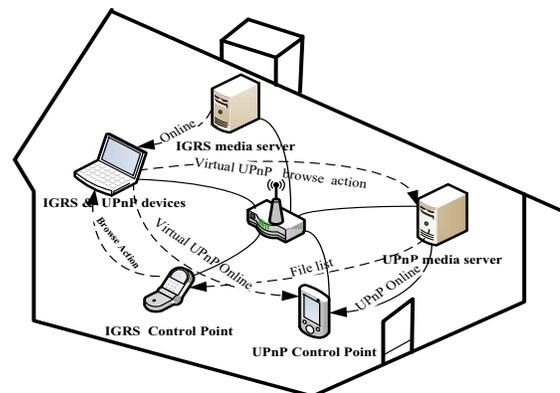
Figure5. Devices interaction basing on agent model framework
