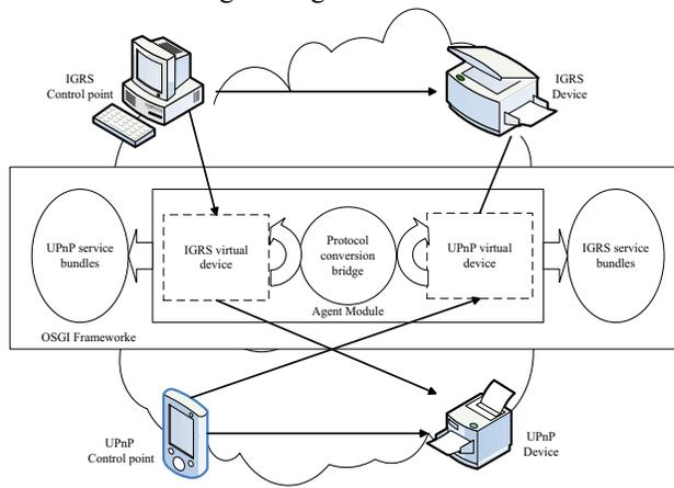
Figure2. Schematic diagram of interconnection between IGRS device with UPnP device through the agent module
