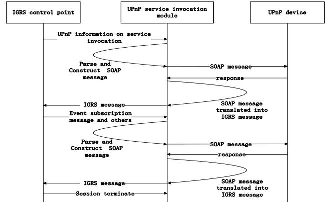
Figure4. workflow of UPnP service call module
