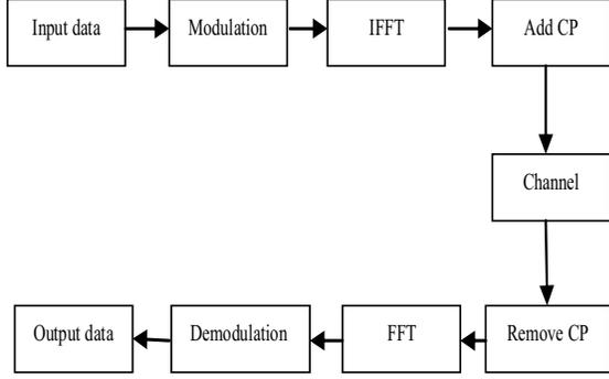
Fig. 1: Block diagram of OFDM system
