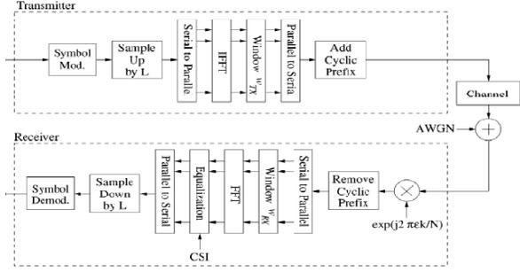
Fig. 2 block diagram of ICI SC with windowing [9]
