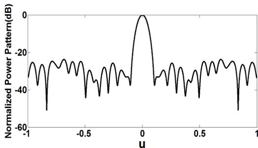
Fig. 3: Normalized power pattern for 34 elements linear array with SLL= -30 dB and single wide null of specified depth is -70dB from 3400 to 3600 FFT point when element 2, 6, 29, 32 are failure
