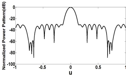
Fig. 4: Corrected Normalized power pattern for 34 elements linear array with SLL= -30 dB and single wide null of specified depth -70dB from 3400 to 3600 FFT point when element 2, 6, 29, 32 are failure.
