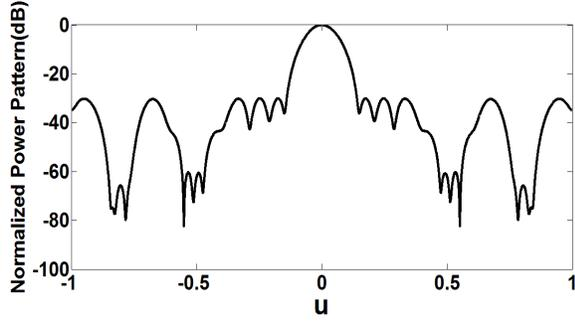
Fig. 7: Corrected Normalized power pattern for 34 elements linear array with SLL=-30 dB and dual wide nulls of specified depths is -70dB from 3000 to 3200 and 3600 to 3800 FFT point when element 2. 6. 29. 32 are
