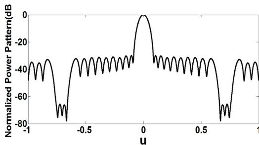
Fig. 2: Normalized power pattern for 34 elements linear array with SLL= -30 dB and single wide nulls of specified depth is -70dB from 3400 to 3600 FFT point
