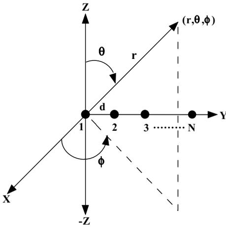
Fig.1. Geometry of an N-element linear array along the Y- axis
