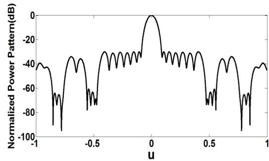
Fig. 5: Normalized power pattern for 34 elements linear array with SLL= -30 dB and dual wide nulls of specified depths is -70 dB from 3000 to 3200 and 3600 to 3800 FFT point
