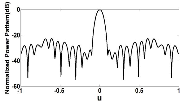
Fig. 6: Normalized power pattern for 34 elements linear array with SLL= -30 dB and dual wide nulls of specified depths is -70dB from 3000 to 3200 and 3600 to 3800 FFT point when element 2, 6, 29, 32 are failure
