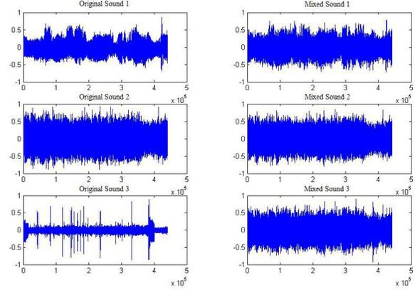
Fig. 1 Original Sound Signal and Mixed Sound Signals
