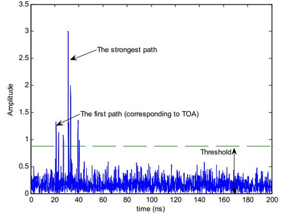
Fig. 1. The received UWB signal under dense multipath and Weibull noise.
