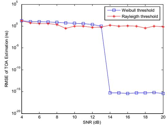
Fig. 2. RMSE v.s. SNR for TOA estimation using two methods
