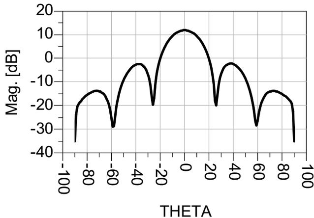
Fig. 13. Gain of 4×1 antenna array
