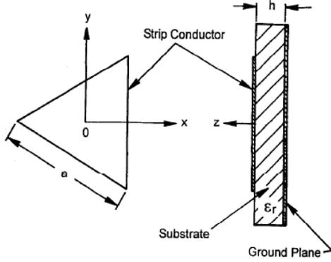
Fig. 1. Geometry of an equilateral triangle microstrip antenna
