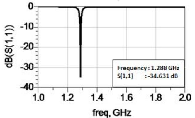
Fig. 5. Return loss of single element antenna
