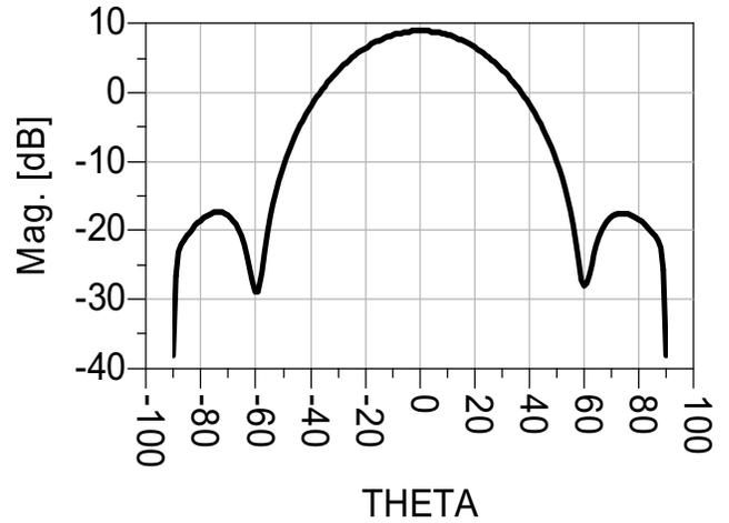
Fig. 10. Gain of 2x1 antenna array
