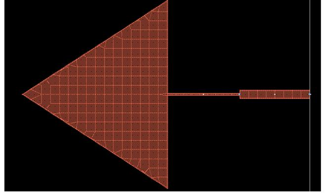
Fig. 2. Single element equilateral triangular patch antenna
