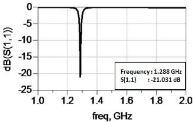
Fig. 8. Return loss of 2x1 antenna array
