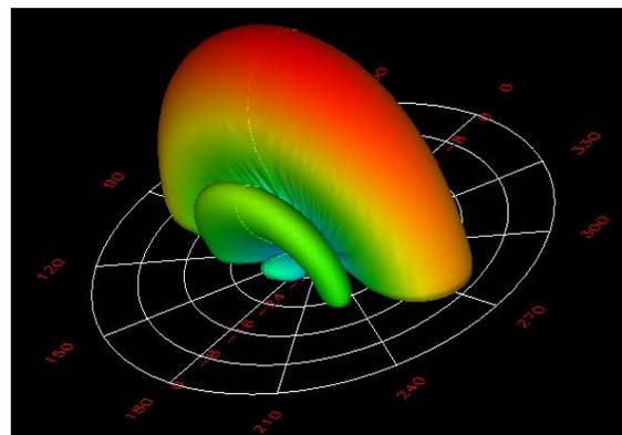
Fig. 12. 3D Radiation pattern of 4x1 antenna array
