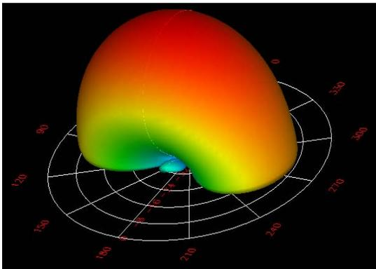
Fig. 9. 3D Radiation pattern of 2x1 antenna array
