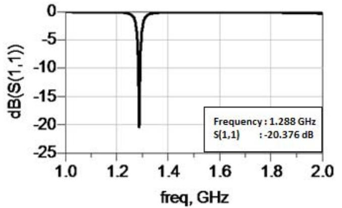
Fig. 11. Return loss of 4x1 antenna array
