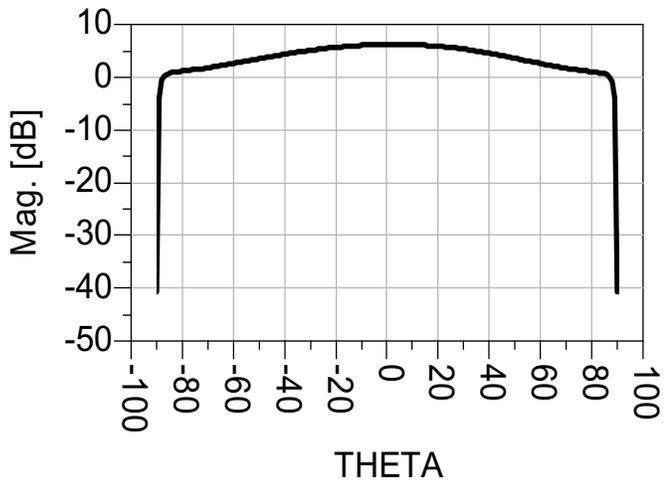
Fig. 7. Gain of single element antenna
