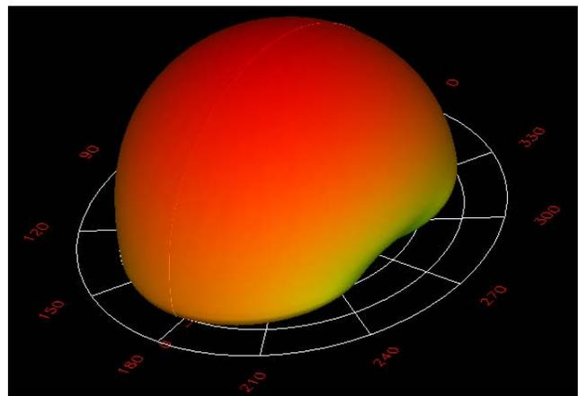
Fig. 6. 3D Radiation pattern of single element antenna
