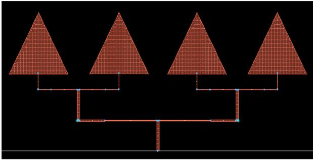
Fig. 4. 4×1 patch antenna array
