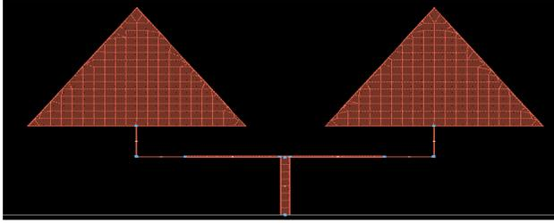
Fig. 3. 2×1 patch antenna array
