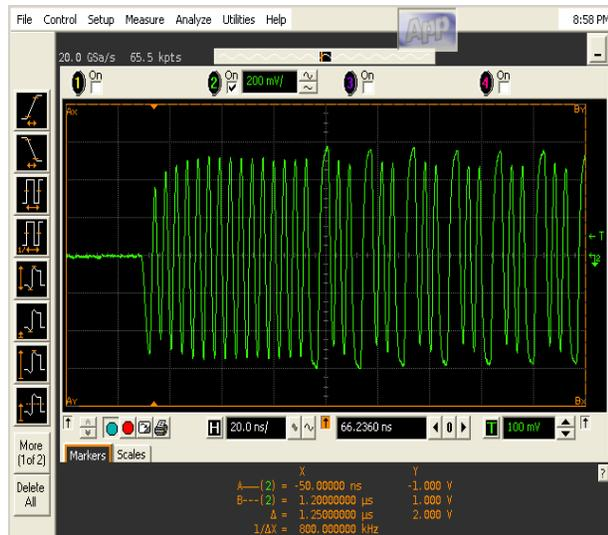
Fig. 4. (b) HS transmit differential data after debugging.
