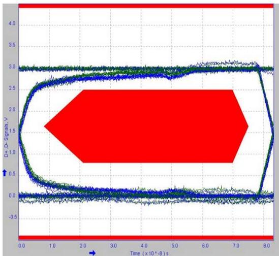
Fig. 2. (b) Passing FS eye diagram after debugging and fix
