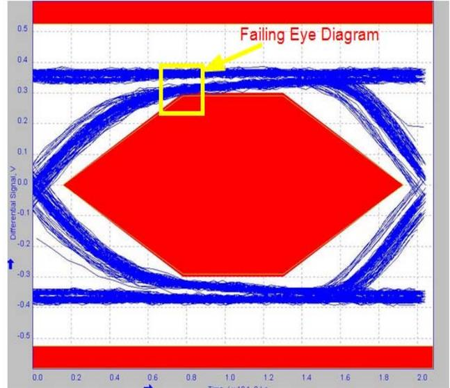
Fig. 3. (a) Failing HS Eye Diagram.
