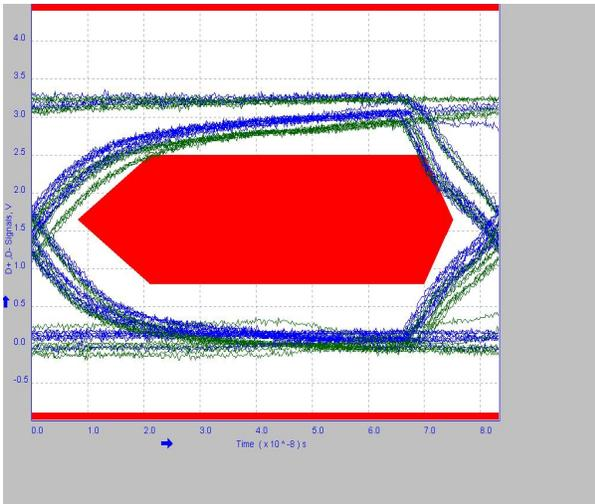
Fig. 2. (a) FS eye diagram failure.
