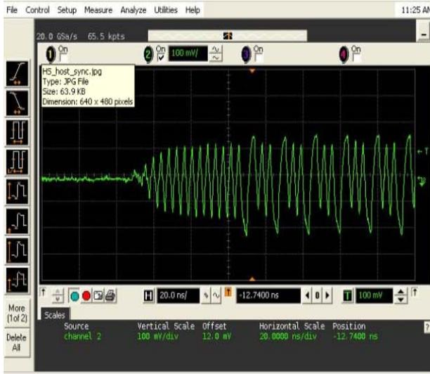
Fig. 4. (a) HS transmit differential data before debugging.
