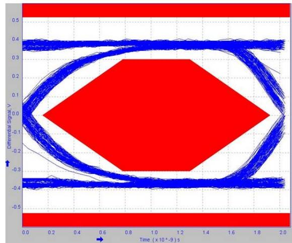
Fig. 3. (b) Passing HS Eye Diagram after debugging.
