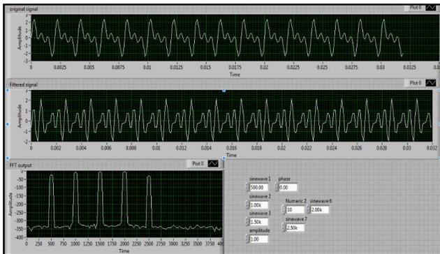
Fig. 8. Front panel of design of IIR filtering system in LabVIEW
