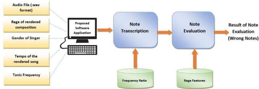
Fig. 1. Architecture of Proposed System
