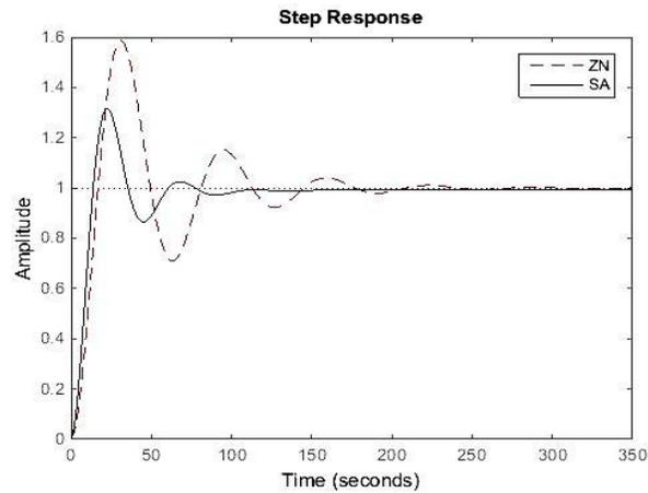
**Fig. 4** Comparison of ZN and SA based set-point tracking responses
