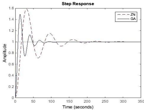
**Fig. 5.** Comparison of ZN and GA based set-point tracking responses
