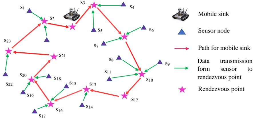
**Fig. 2.** A sub graph of WSN having 23 number of sensor nodes. Out of 23 11 sensor nodes act as RP.
