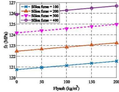
Fig. 5: Variation of compressive strength as a function of Fly Ash and Silica Fume
