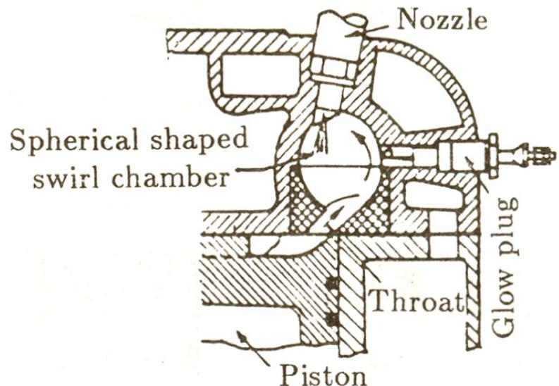
be reduced by employing a heat insulated passage. This type of combustion chamber finds its application where fuel quality is difficult to control, where reliability under adverse conditions is more important than fuel economy. The use of single hole of larger diameter for the fuel spray nozzle is often important consideration for the choice of swirl chamber engine.
