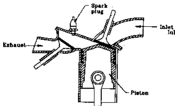
F – head used in Willeys jeep.
