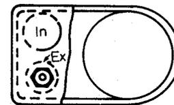
**RICARDO'S TURBULENT HEAD- SIDE VALVE COMBUSTION CHAMBER (VTU July 06)**
