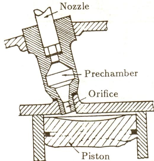
**Fig.10.21** Precombustion Chamber
