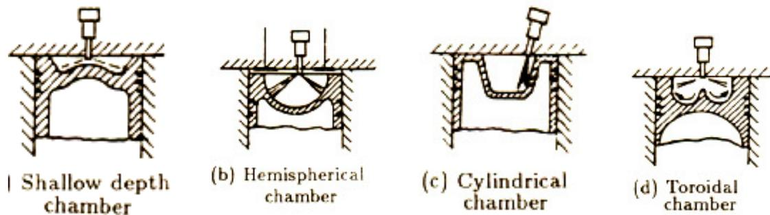
Shallow Depth Chamber: In shallow depth chamber the depth of the cavity provided in the piston is quite small. This chamber is usually adopted for large engines running at low speeds. Since the cavity diameter is very large, the squish is negligible.
