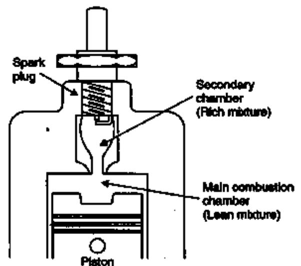
Fig. 5.23. Divided combustion chamber.
