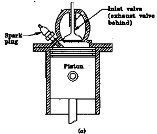
Wedge Type Combustion Chamber. In this design slightly inclined valves are used. This design also has given very satisfactory performance. A modern wedge type design can be seen in for Plymouth V-8 engine. It has a stroke of 99 mm and bore of 84mm with compression ratio 9:1
