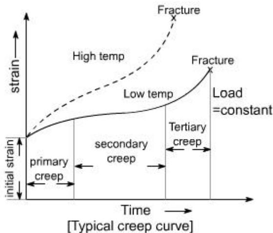
The general form of  $\epsilon$  Vs  $t$  graph or creep curve is shown below for two typical operation conditions, In each case the curve can be considered to exhibit four principal features
