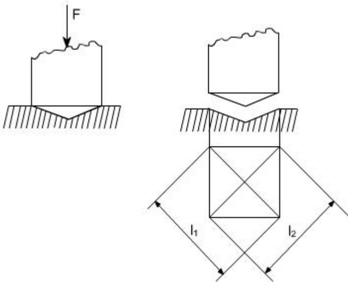
In the Vicker Test the indenters of pyramidal or conical shape are used & this overcomes the disadvantage which is faced in Brinell test i.e. as the load increases, the geometry of the indentation's does not change
