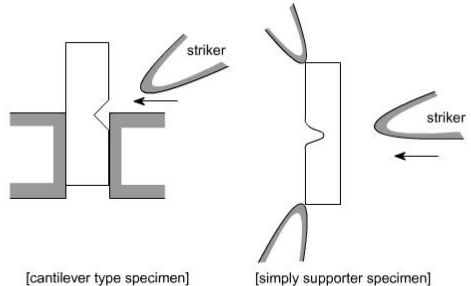
The specimen may be of circular or square cross – section arranged either as a cantilever or a simply supported beam.
