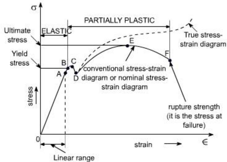
**Nominal stress – Strain OR Conventional Stress – Strain diagrams:**
