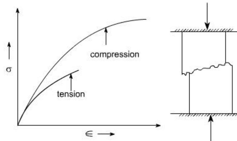
Brittle materials in compression behave elastically up to certain load, and then fail suddenly by splitting or by cracking in the way as shown in figure. The brittle fracture is performed by separation and is not accompanied by noticeable plastic deformation.
