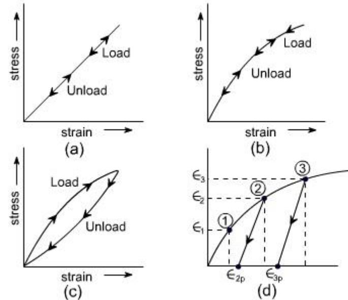
Many engineering materials behave as indicated in Fig(a) however, some behaves as shown in figures in (b) and (c) while in elastic range. When a material behaves as in (c), the  $\sigma$  vs  $\epsilon$  is not single valued since the strain corresponding to any particular '  $\sigma$  ' will depend upon loading history.
