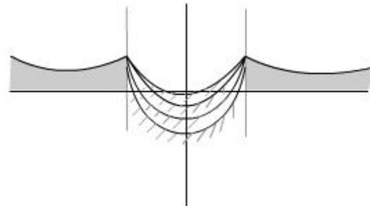
Here what we mean is that the geometry of the impression should not change w.r.t. load, however the size of impression may change.
