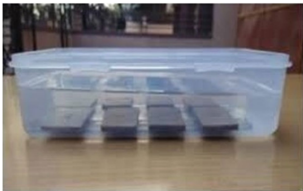
Fig. 4 Set up for the water absorption test
